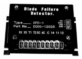
The Stamford Diode Failure Detector (DFD) is suitable for use with all Stamford Generators. It senses the level of ripple current in the exciter output to provide indication of a failed diode, either short or open circuit.
