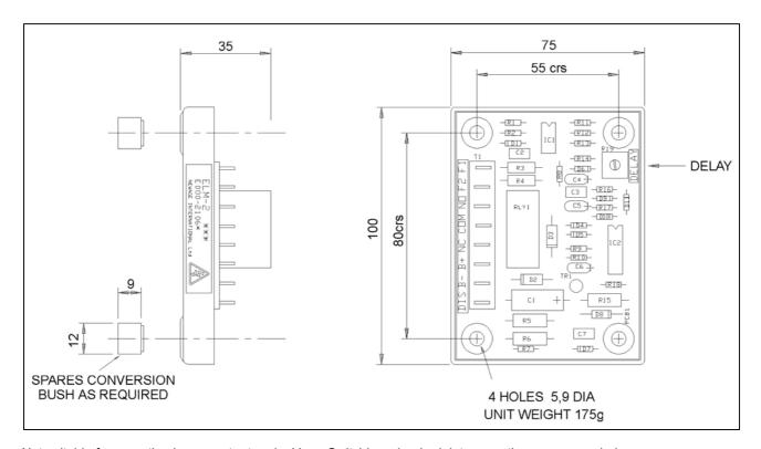
Not suitable for mounting in generator terminal box. Switchboard or bedplate mounting recommended.
