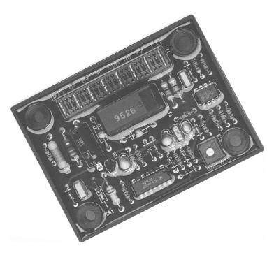
A loss of generator excitation during parallel operation will result in heavy circulating currents, pole-slipping (loss of synchronisation) and torque/current surges and oscillation. The Stamford Excitation Loss Module monitors the generator AVR output and signals any sustained interruption to an integral relay to initiate an indication/alarm.
