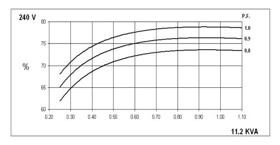
Winding 06 Locked Rotor Motor Starting Curve
