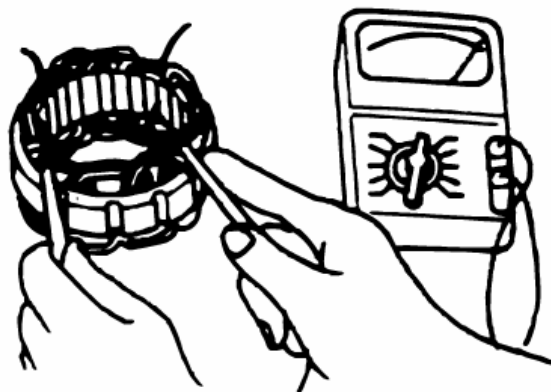
Inspecting the stator coil
