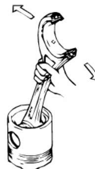
Replacing connecting rod bushing
