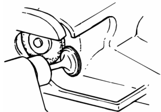
Refacing a valve
