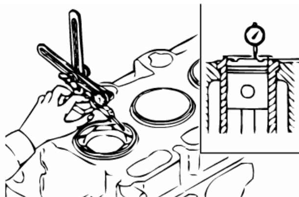
Measuring piston protrusion
