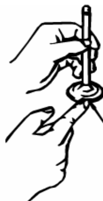
Coating valve with lapping compound
