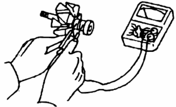
Inspecting the rotor coil
